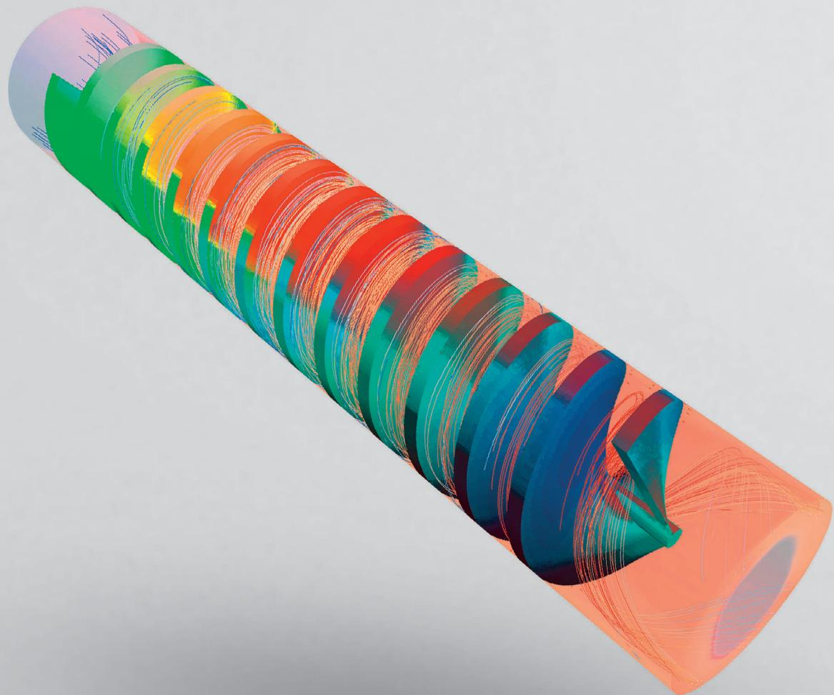
OpenFoam based finite-volume simulation of conjugate heat transfer between a homogeneously heated spiral and an air steam. The air stream expands and doubles its Viscosity within 10cm.
