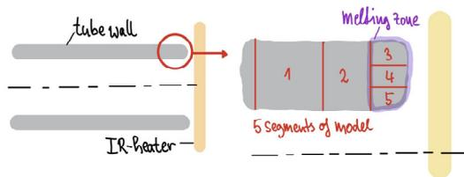
Fig. 1: The model is based on the discretisation of the pipe ends into only five segments.
