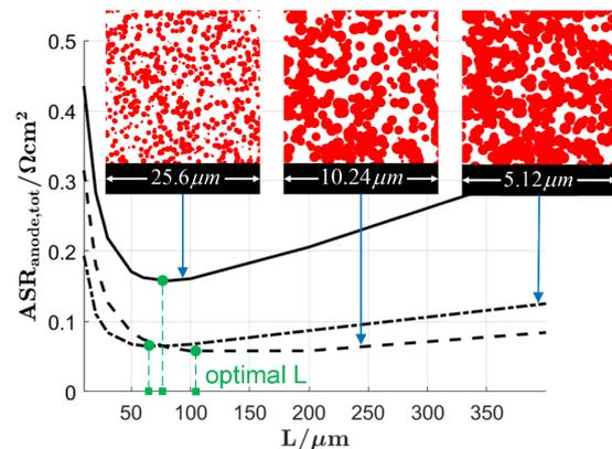
Fig. 2: Area specific resistance (ASR) of CGO-anodes for different microstructures as a function of the anode layer thickness  $L$ .
