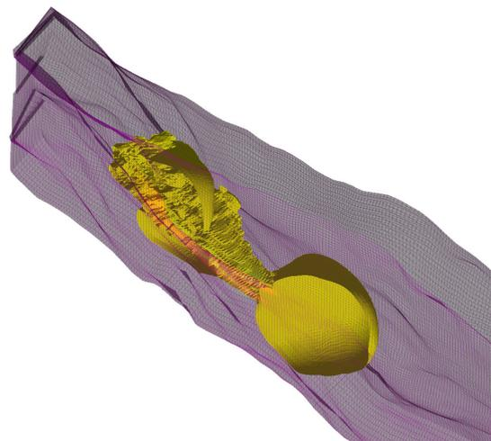
Figure: Simulated avalanche pressure front (view from below).
