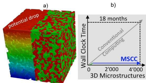
Figure 1: a) Virtual LST/CGO structure of an SOFC anode with computed potential drop, b) comparison of computation time with classical and MSCC approach.
