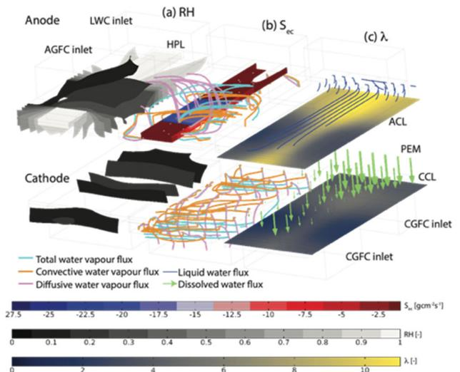
Figure 2: Water management at anode side (top) and cathode side (bottom). (a) Relative humidity (RH). (b) Evaporation rate and streamlines of water vapour flux. (c) Streamlines of liquid water flux and dissolved water flux, water content dissolved in the membrane ( $\lambda$ ).
