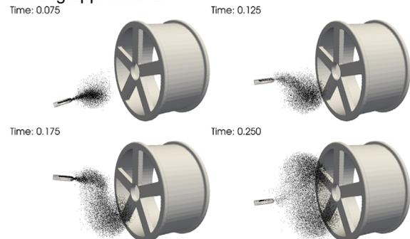
Figure 1: Snapshots from a simulation of a car rim being coated with a pistol with combined translational and rotational motion.
