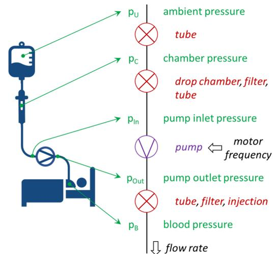
Figure 2: Model of the infusion system with pump and various components.
