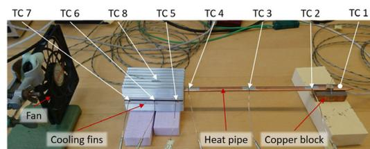
Fig. 1: Test setup for measuring the eff. thermal conductivity of a heat pipe; copper block with heating cartridge (right), heat pipe (centre), cooling fins (left), fan for forced convection (left); designations of the T-measuring points above the diagram.
