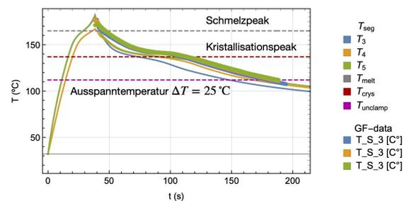
Fig. 2: Validation of the weld temperatures predicted by the model via welding tests with T-sensors placed in the weld seam.
