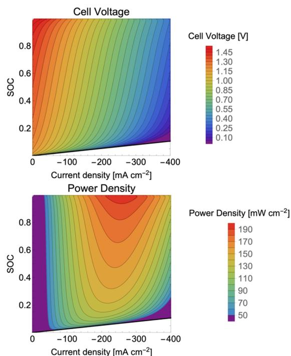
Figure 1: Predicted cell voltage (above) and power density (below) of an electrochemical cell using the 0-D U-I-SoC model.
