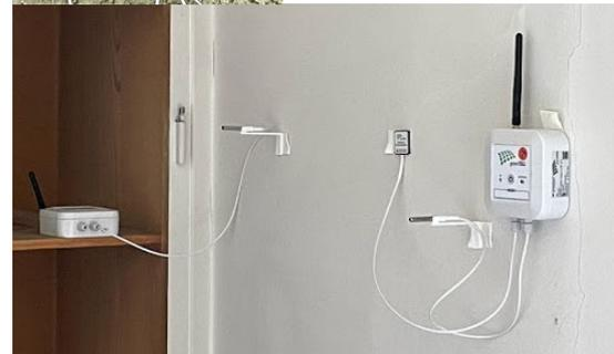
Fig. 2: On the inside of the wall, in the heated zone of the building, surface temperature and air temperature are also measured. In addition, the heat flow and air humidity are recorded. The data is transmitted wirelessly to a server via a base station and processed in a cloud application.
