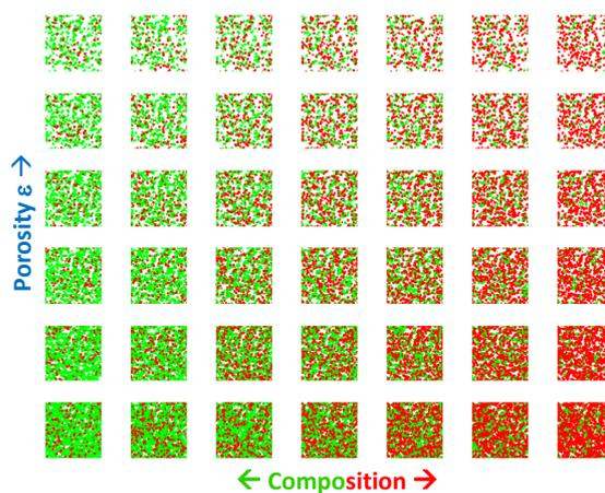
Figure 2: Example of a small parameter study for different porosities and compositions of an LST/CGO anode.
