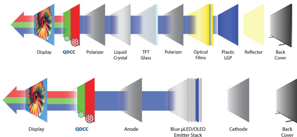
Fig. 1: QD film in an LCD screen (top) and in an OLED screen (bottom). Source: Nanosys Inc..
