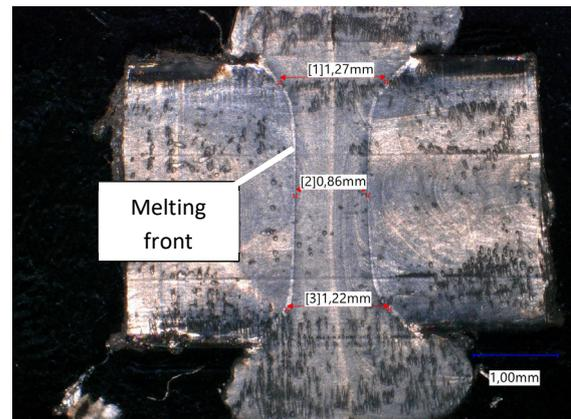
Fig. 2: Microtome section of a weld seam under a light microscope.
