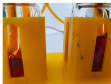
Figure 3: Picture of positive (left) and negative (right) reservoirs after cycling. The height was initially equal.
