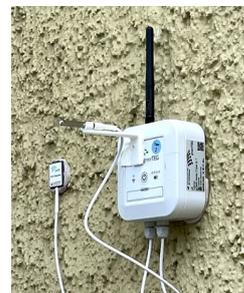
Fig. 1: Measuring system for determining the heat transfer coefficient (U-value). The installation was carried out for test purposes on the "TK" building on the campus of the School of Engineering of ZHAW. The figure shows a temperature measurement on the outer wall. It is important to note that wall surface temperature and air temperature are recorded separately.
