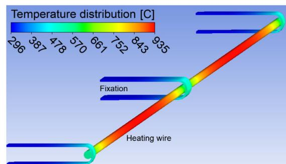
Fig. 3: Temperature distribution on the heating wire surface.
