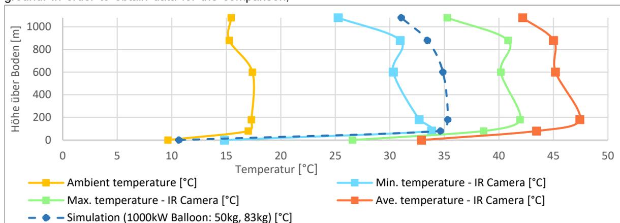
Fig. 1 Comparison of the ambient temperature measured with a temperature sensor in yellow, the minimum/maximum temperature measured with the IR camera in blue and orange respectively, the average value in green and the simulated envelope temperature in dark blue. For the simulation, a burner power of 1'000 kW, a mass of 50 kg and a load of 83 kg is used.
