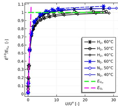
Figure 2: Normalized evaporation rates as a function of normalized gas velocities. Normalization is based on convective and diffusive transport limitations at low and high gas velocities, respectively.
