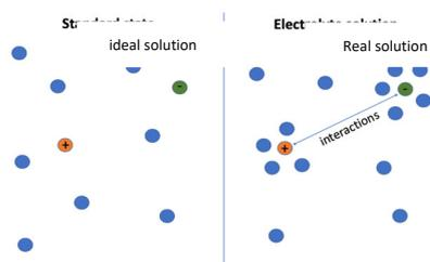
Figure 1: Ideal solution (left): interactions are neglected / Real solution (right): electrostatic and short-range interactions affect electrolyte properties.
