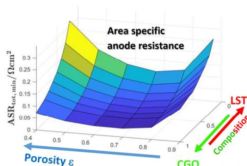
Figure 3: Resulting area specific anode resistance as a function of porosity and composition of an LST/CGO anode.
