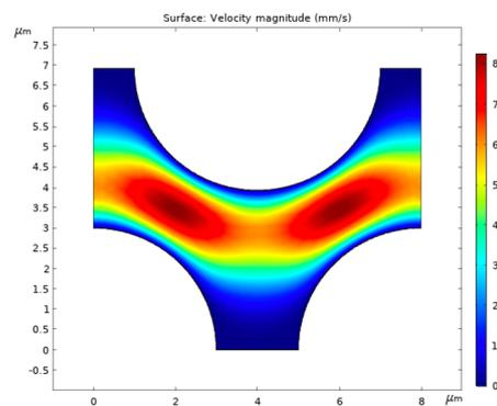
Figure 1. Geometry of the proposed periodic cell used to study combined macroscopic flow and mass transport phenomena (liquid velocity magnitude contours are superimposed). White semi-circles are the cross-section of periodic electrode matrix (fibres).
