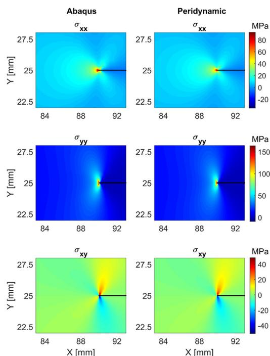
Fig 2: Comparison of the stresses simulated in a plate with a slit crack using Abaqus finite element with those using bond-based peridynamics
