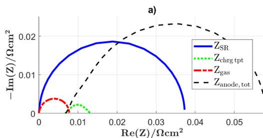
Fig. 1: Deconvolution of the simulated anode EIS-spectra:  $Z_{SR}$  = hydrogen oxidation surface reaction impedance,  $Z_{chrg\ tpt}$  = charge carrier transport imped.,  $Z_{gas}$  = gas imped.,  $Z_{anode,tot}$  = total anode imped.
