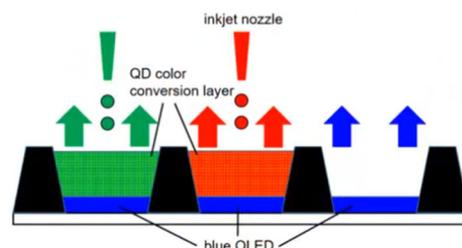
Fig. 2: Schematic representation of an OLED pixel with a QD film..
