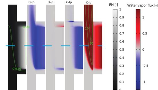
Figure 3: 2-D model results at high  $U/U^0$ : relative humidity RH (left) and diffusive (D) and convective (C) through-plane (tp) and in-plane (ip) normalized water vapor flux.
