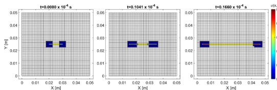
Fig. 2: Adaptive relocation of multiple PD patches for a single crack in the medium.
