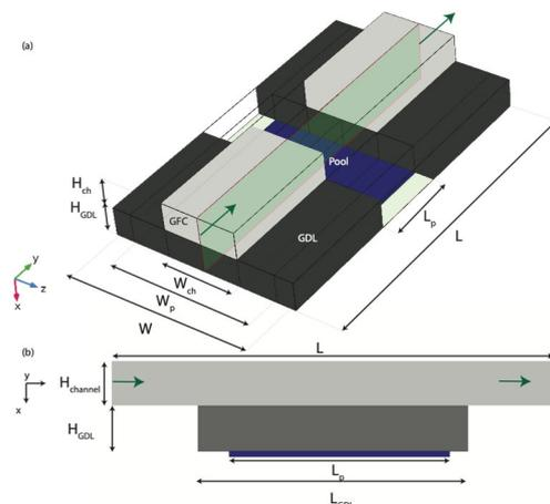
Figure 1: Setup of (a) 3-D and (b) 2-D model of evaporation in a GDL in contact with a gas flow channel.
