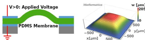
Fig. 2: computational prediction of PDMS buckle under voltage.
