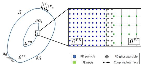
Fig. 2: Introduction of ghost particles and discretization near the coupling interface
