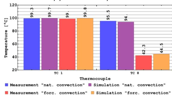
Fig. 3: Validation of the CFD model for 100°C heating temperature and 23°C room temperature with and without fan operation. TC 1 indicates the measuring point on the heater, TC 8 that on the cooling fins.
