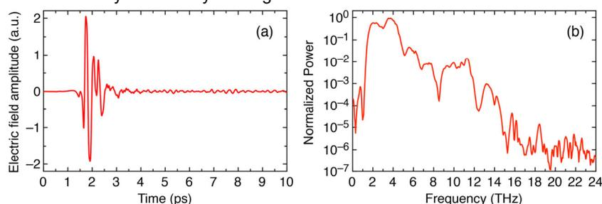
Fig 2.: THz time-domain signal (a) and the corresponding power spectrum (b) of the THz setup based on organic crystals: The aim of this project is to reduce the modulation of the signal seen in (b) to achieve a flat spectral response over the whole frequency range.
