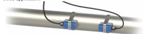
Fig. 3: The ultrasonic flowmeter determines the velocity of heating water in a pipe, without having to cut any it open. Together with two temperature measuring points, it is then possible to determine the heat flow transported from one part of the system to another.
