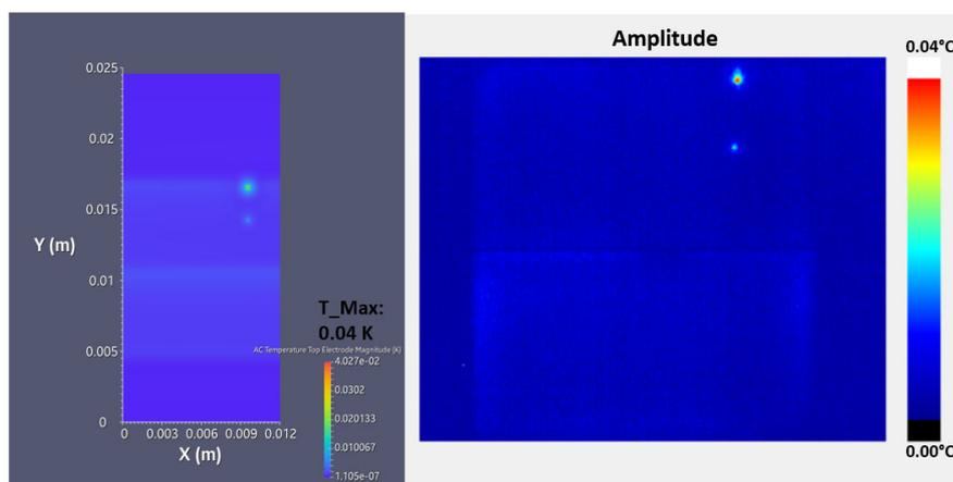
Figure 1: Simulated SS-DLIT amplitude image of a perovskite dual cell showing a temperature increase at the shunts and the interconnection. The SS-DLIT amplitude measurement is shown on the right, displaying two hot spots in the upper cell as well, which cause losses during operation.
