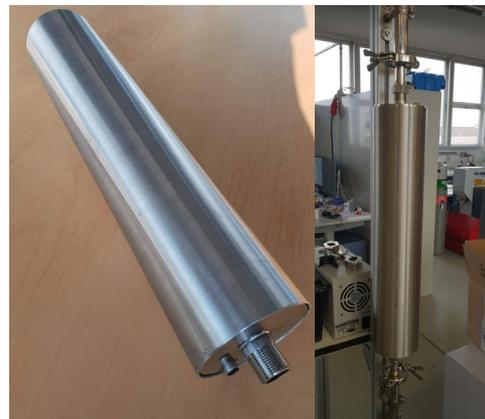
Figure 1: DN20 tubular resonator (left), DN20 tubular resonator operating in an experimental flow loop.
