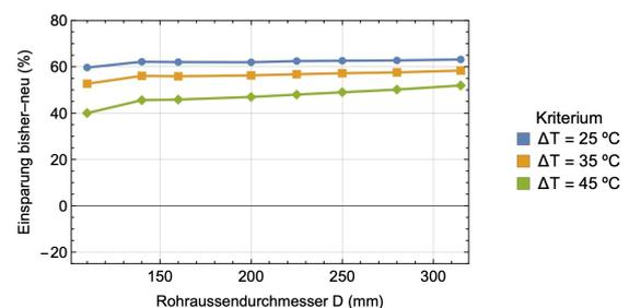
Fig. 3: Shortening of the welding time of plastic pipes when using the newly developed model, which simulates the behaviour of the weld seam temperatures and thus predicts the optimum unclamping time of the welded pipes.
