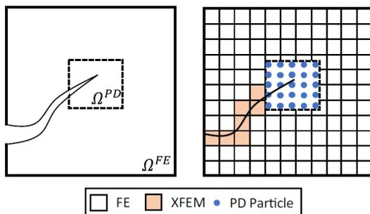
Fig. 1: Schematic of the PD-XFEM coupling.
