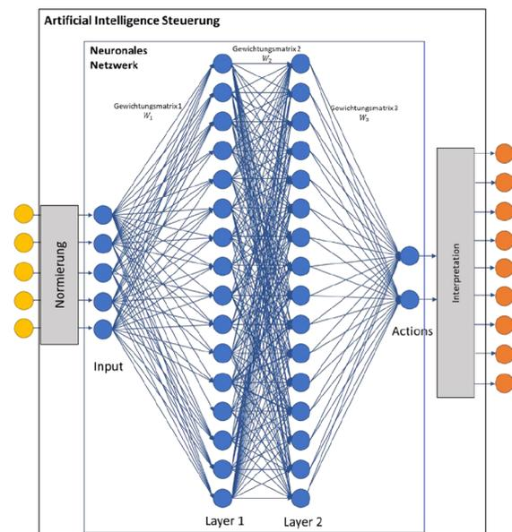
Figure: Neural network used in [1]. Input datapoints (signals from sensors) are symbolized with yellow circles, output data (signals to actors) are shown by orange circles.
