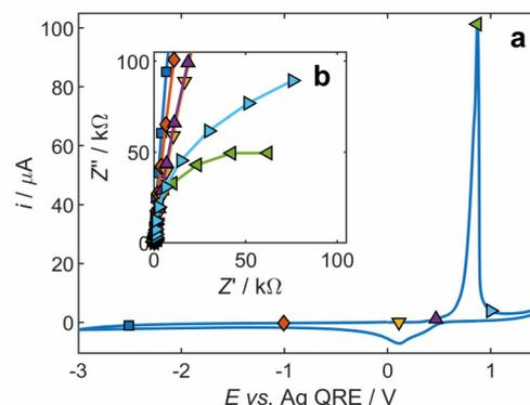
Figure 2: **a**: Cyclic voltammogram measured on an NPB thin film. The impedance spectra shown in **b** were obtained at different potentials marked by symbols in **a**.
