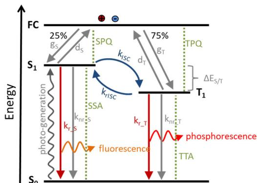
Figure 1: General exciton and charge transfer processes. FC denotes the free carriers, S1 the singlet, T1 the triplet exciton, and S0 the ground state.
