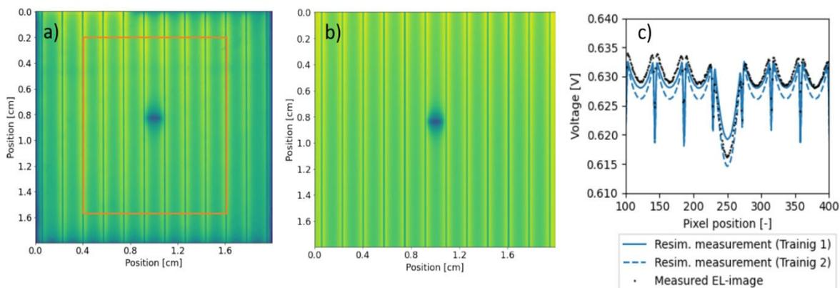
Figure 1: Measured (a) and with Laoss simulated (b) EL image of a silicon solar cell with an intentionally induced shunt and metal fingers (vertical lines). A horizontal cross-section of the resulting junction voltage, when the device is resimulated with the parameters extracted from the CNN, trained with two different training sets is shown in c).
