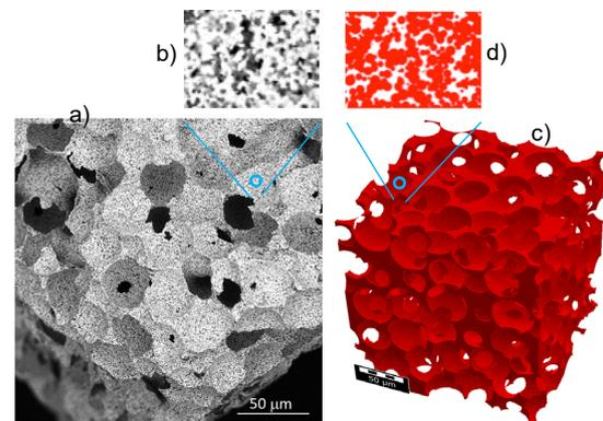
Figure 1: Microscopy image of the ceramic multiscale structure of the mesoscale a) and microscale b). Virtual reconstruction of the mesoscale c) and microscale of the multiscale filter structure using GeoDict.
