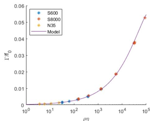
Figure 2: Bandwidth divided by the resonance frequency ( $\Gamma/f_0$ ) vs. the viscosity density product  $\rho\eta$  for different fluids and the numerical prediction.
