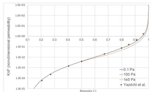
Figure 2. Validation of the model using a study of Yazdchi et al. [3] as a benchmark.
