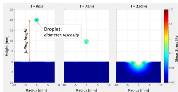
Figure 1: Side view on splashing test-case with falling droplet (top) and resting fluid (bottom) in a cylindrical domain. Time progresses from left to right; color indicates magnitude of azimuthal shear stress average.
