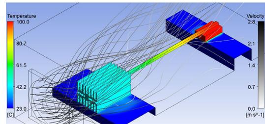
Fig. 2: Representation of the CFD simulation results with 100°C heating temperature and forced convection generated by a PC fan. The surface temperatures are shown in colour and the air flow in black and white.
