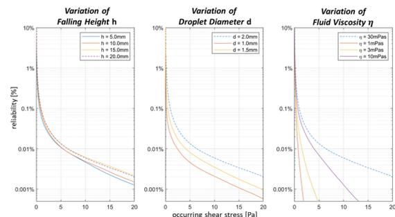
Figure 2: Reliability function (probability of occurrence of a certain shear stress) used to compare the effect when changing one of the parameters. Left: marginal effect when varying the falling height; Middle: medium effect when varying droplet diameter; Right: large effect when varying fluid viscosity.
