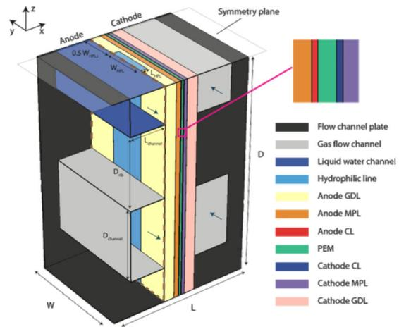
Figure 1: 3-D model setup. Anode flow field with one gas and liquid water channel, respectively, a cathode flow field with two gas channels. The membrane electrode assembly includes the hydrophobic anode gas diffusion layer with one hydrophilic line.
