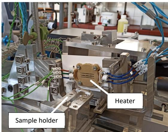
Fig. 1: Test bench for welding plastic samples.
