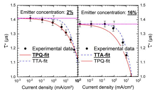
Figure 2: Excited states lifetime data for increasing current densities of an OLED with an emitter concentration of 2% (left) and 16% (right). Fit to experimental data clearly shows that the decrease at higher currents is better described by TPQ for the case with 2%, and by TTA for the case with 16%.
