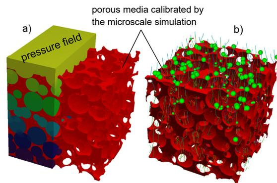
Figure 2: a) Simulation of the pressure drop in order to determine the permeability and b) filtration simulation to determine the filter efficiency using GeoDict. The microscale of the structure is respected by calibrating its permeability and filter efficiency statistics in the porous media of the mesoscale structure.
