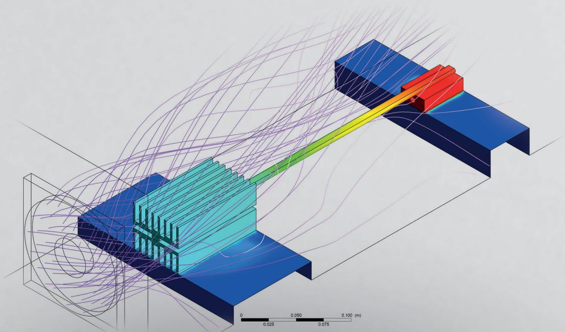
CFD simulation illustration of a heat pipe with 100 °C heating temperature and forced air cooling via aluminum cooling fins.
