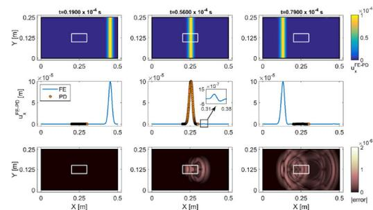
Fig. 3: Pulse propagation in the coupled FE-PD model captured at three-time instants.
