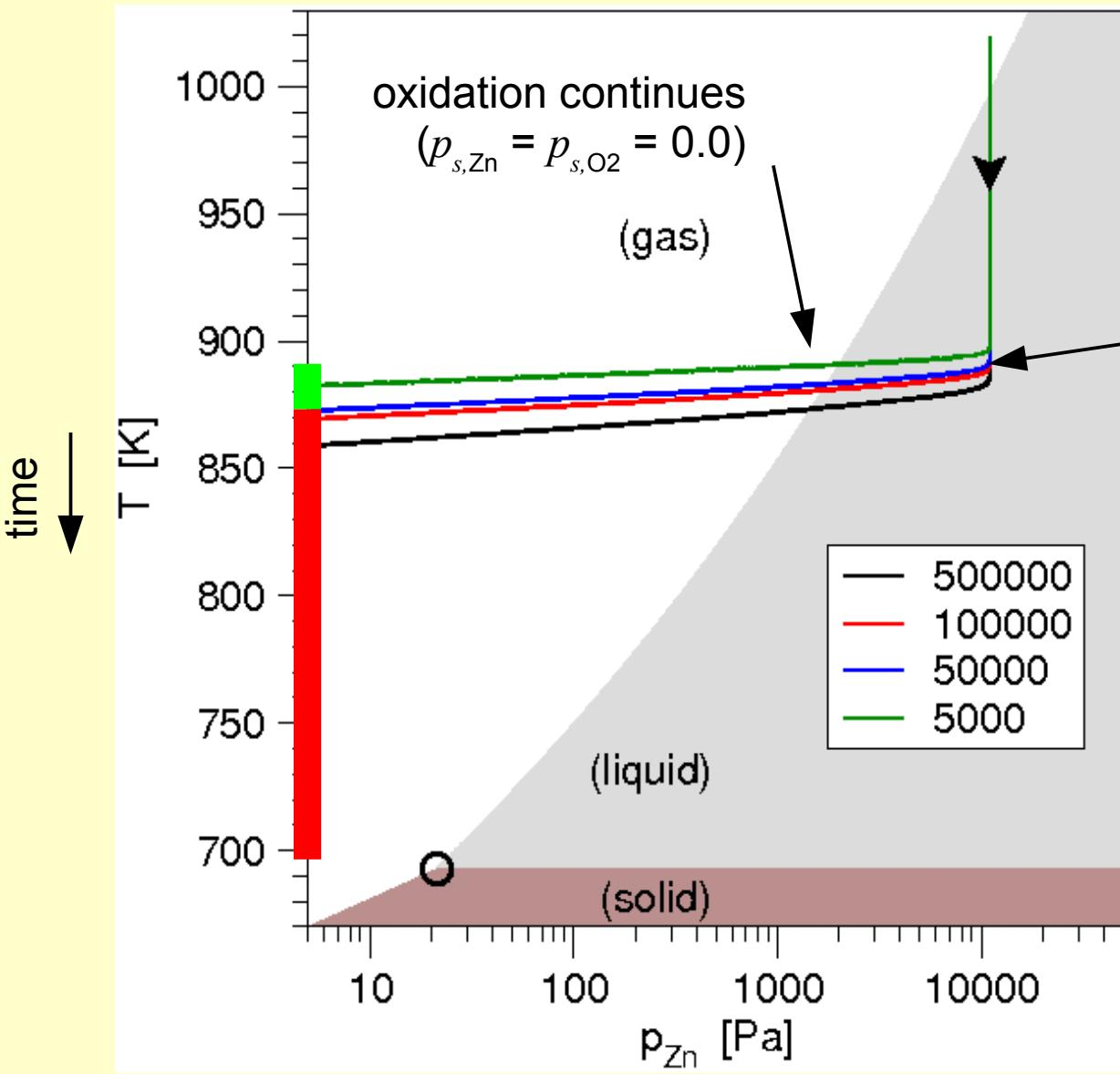
increased quench rate results in increased nucleation super saturation and nucleation rate
