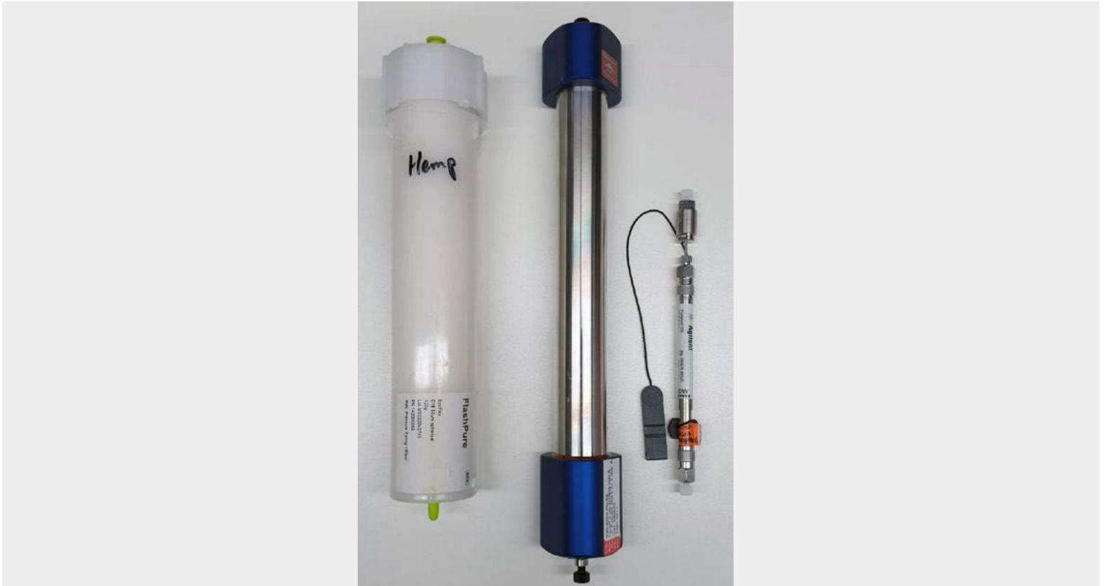
Fig. 3: (left to right) Column for flash chromatography, preparative chromatography and HPLC-MS
