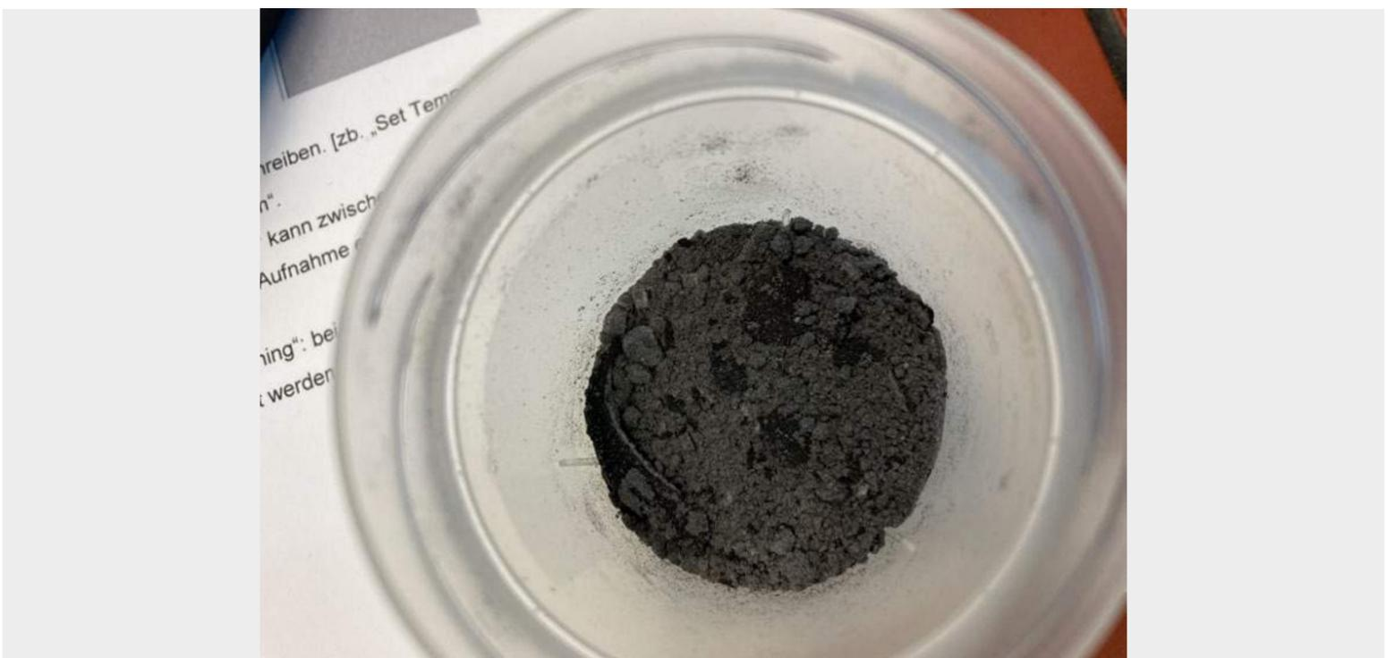
Fig. 2: Biochar made by wheat straw
