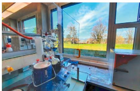
Fig. 1: Set up of Safe-distillation used for aroma extraction at Campus Grentel
