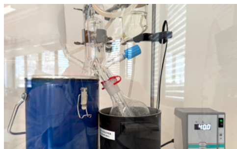
Fig. 2: Solvent-assisted flavour evaporation (SAFE) apparatus used for the isolation of volatile aroma compounds from the product
