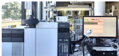
Fig. 1: Gas chromatography-olfactometry-mass spectrometry (GC-O-MS) system used in aroma extract dilution analysis (AEDA)
