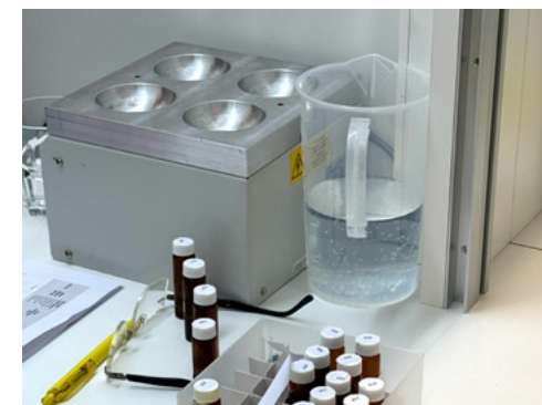
Fig. 1: Example of orthonasal evaluation of developed samples by the Swiss Olive Oil Panel (SOP), prepared in an amber glass vial with a PE/PTFE liner cap under standard test conditions
