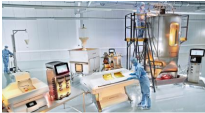
Figure 1: SUS often used in upstream processing (with kind permission from Sartorius Stedim Biotech)
