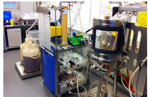
Figure 2: Experimental set-up of an upstream perfusion process executed in Sartorius Stedim's BIOSTAT STR 50L with a hollow fiber cartridge from GE Healthcare in our lab.
