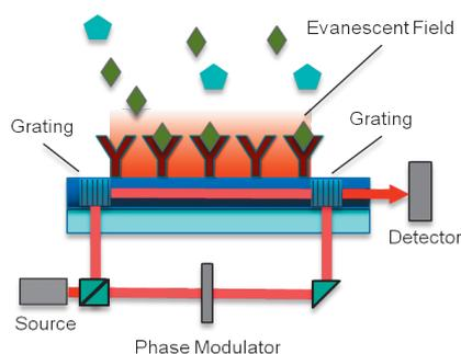
Fig. 1: Structure of the grating-coupled interferometer (l) and sensor with integrated tantalum pentoxide wave guide (r)
