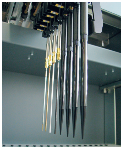
Coated pipetting needles (at rear) and disposable tips (at front) integrated into a robot arm.
