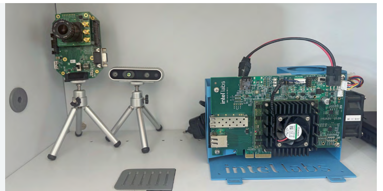
This dynamic vision sensor works like a human retina. Each pixel detects luminance change and sends a small data package to the computer. The neuromorphic computing chip, shown next to the camera, can process exactly such "event-based" information. The left-hand picture provides a schematic representation, while the right-hand picture is a photo of the cameras and the chip in the current prototype version.
