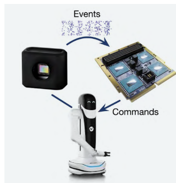
This dynamic vision sensor works like a human retina. Each pixel detects luminance change and sends a small data package to the computer. The neuromorphic computing chip, shown next to the camera, can process exactly such "event-based" information. The left-hand picture provides a schematic representation, while the right-hand picture is a photo of the cameras and the chip in the current prototype version.
