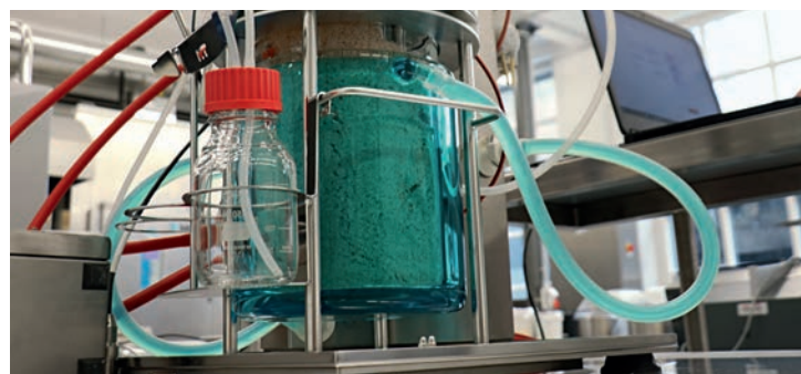
Fig. 1: Fermentation of wheat bran in a solid fermenter to verify the minimum necessary water content which allows metabolic activity of fermentation-relevant microorganisms.
