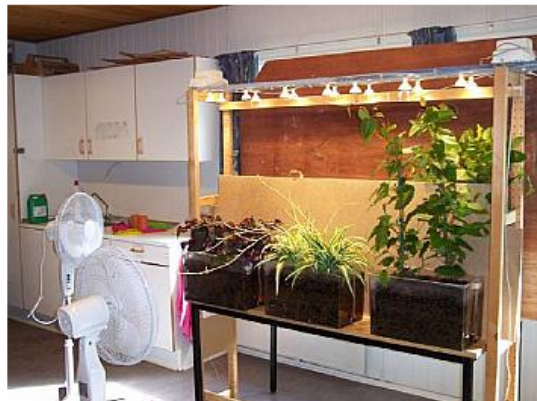
Fig. 1: Setup for the Evapotranspiration experiment in the classroom
