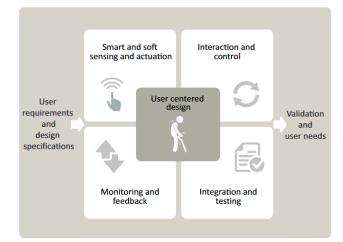
User requirements and design specifications are established before concept technology development commences. The design is realised in the selection of technologies, which are developed based on their ability to deliver the user centered design solution. Finally, the mature prototype will be evaluated in clinical and home trials.
