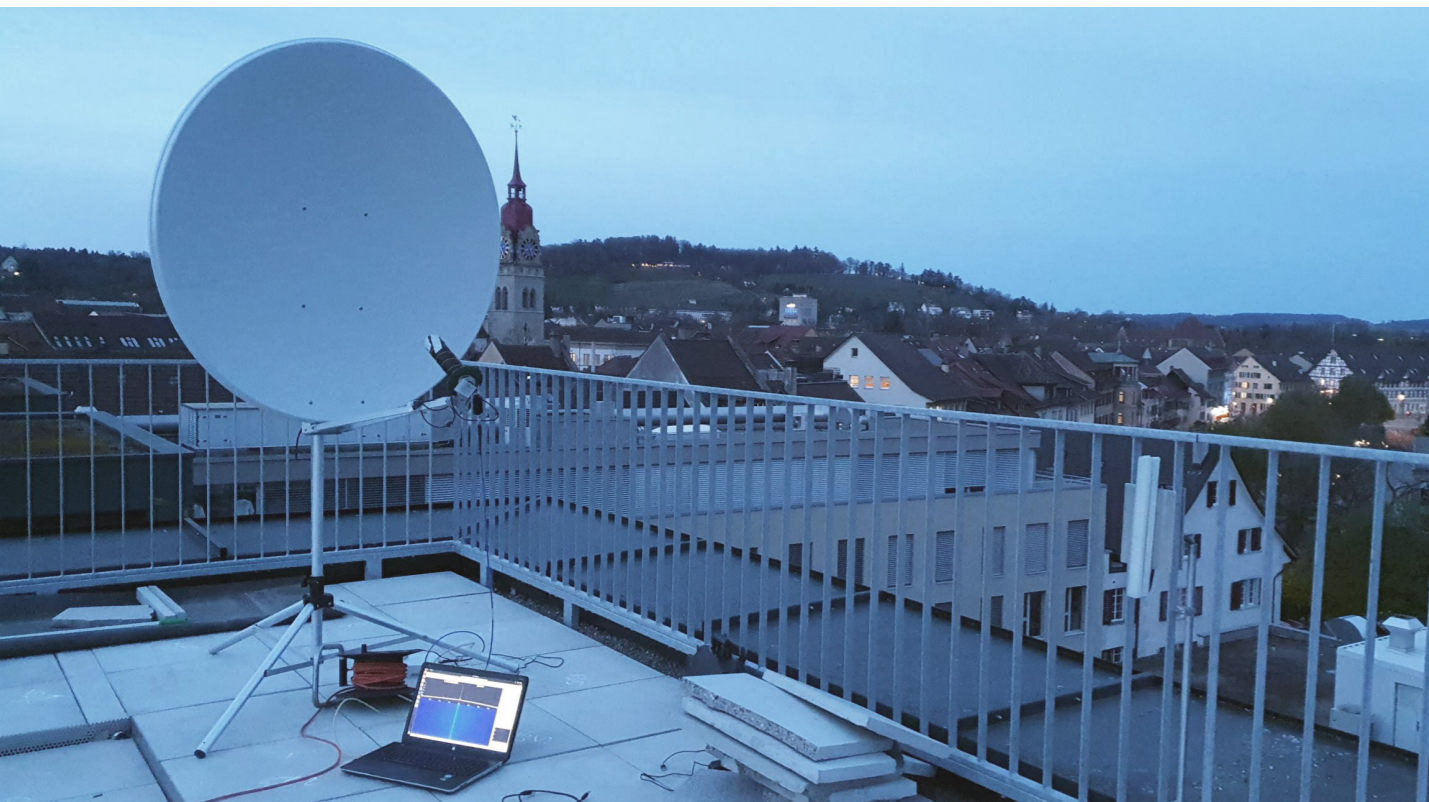
NOAA weather satellite data receiver as part of a bachelor thesis in 2022. The receiver was built using a helical antenna with a parabolic reflector, an RTL2832U Software Defined Radio (SDR) and a GNU Radio based decoding algorithm.
