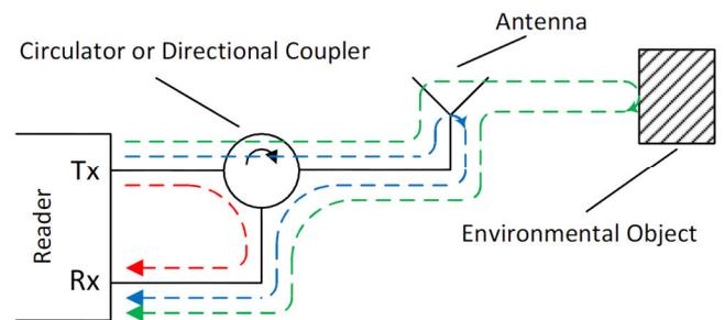
Fig. 1. Tx to Rx carrier leakage paths
