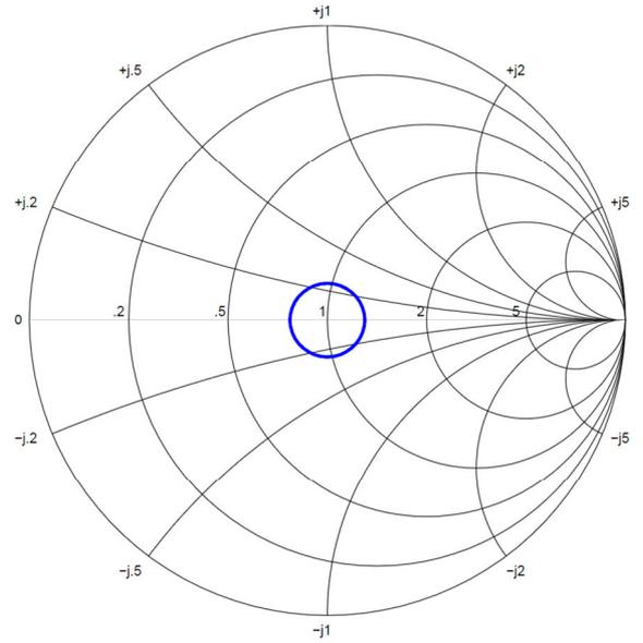
Fig. 3. Impedance area for 18dB antenna reflection loss
