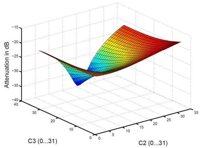
Fig. 7. Tx to Rx carrier attenuation with RL=15dB
