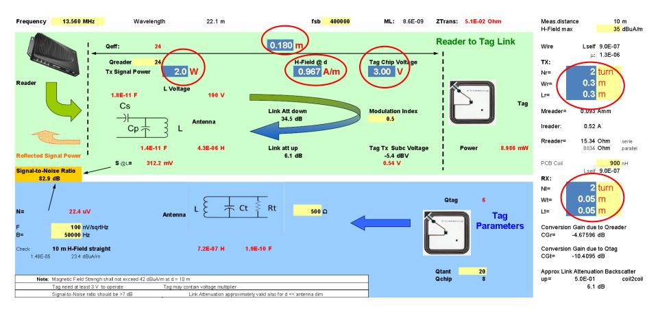
→ Loaded Tag Antenna: Optimum number of turns is 2
