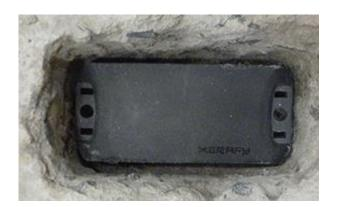
Robust chemically inert tag e.g. Bric from *Xerafy reaches:*
