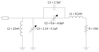
Fig. 8. Implemented impedance network
