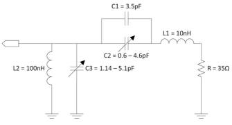
Fig. 4. Simulated impedance network
