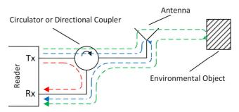
Fig. 1. Tx to Rx carrier leakage paths
