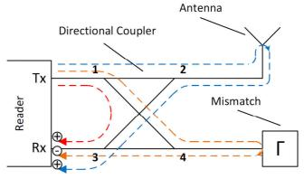
Fig. 2. Principle of the mismatched coupler
