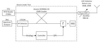
Fig. 10. Measurement setup
