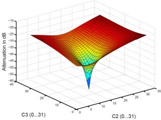
Fig. 6. Tx to Rx carrier attenuation with RL=20dB
