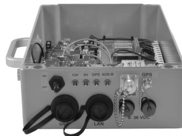
Fig. 2: Mobile MLAT receiver hardware inside a waterproof and shock-resistant housing.
