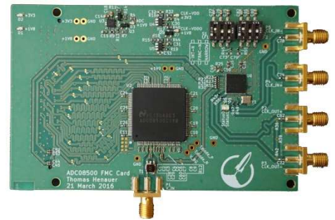
ADC for Multifrequency-GNSS-Rx (BP-Sampling).
