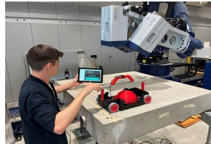
Non Destructive Testing (acoustic)
