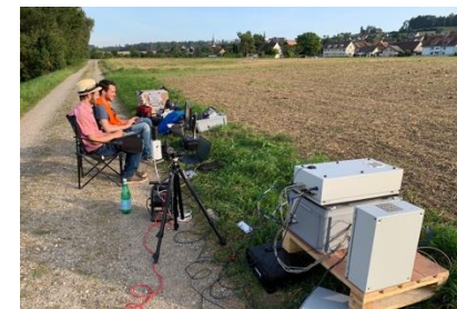
X-Band FMCW Bird Radar (field test, Innosuisse-Project )
