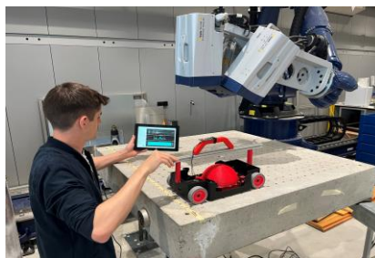
Non Destructive Testing (acoustic)
