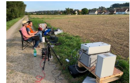
X-Band FMCW Bird Radar (field test, Innosuisse-Project )
