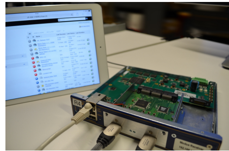
InES Regression Test System based on an embedded system. It is connected over Ethernet to the local network, therefore it is possible to control the tests from any network capable device.
