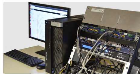
PC based test setup for a high definition video and audio transmission over Ethernet. The test system simulates on the PC all the video/audio sources and sinks as well as an Ethernet network.
