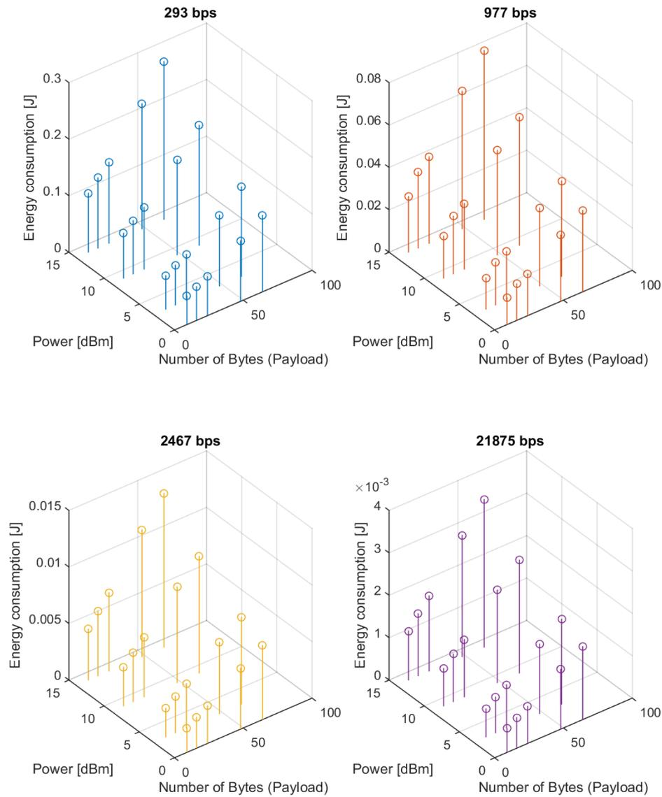
Fig.11 Energy consumption when sending frames of different sizes using LoRa at different baud rates.
