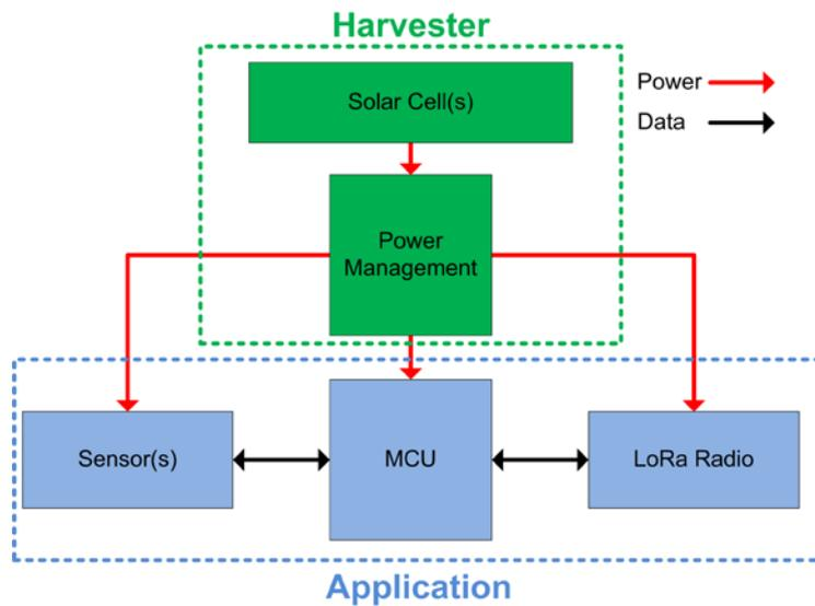
Fig.2 Basic block diagram of the sensing embedded system.
