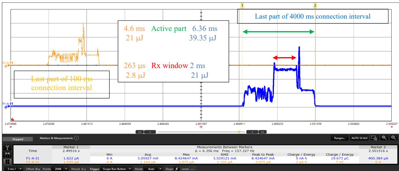
Fig. 15. Effect of clock accuracy on energy. Keep Alive connection of EM9304 SD RC (at 2 V). Zoom on active parts. The Rx window is larger for 4000 ms conn. Interval, compared to 100ms. The RC clock is not very accurate, leading to a higher wait time and more energy for long connection intervals.
