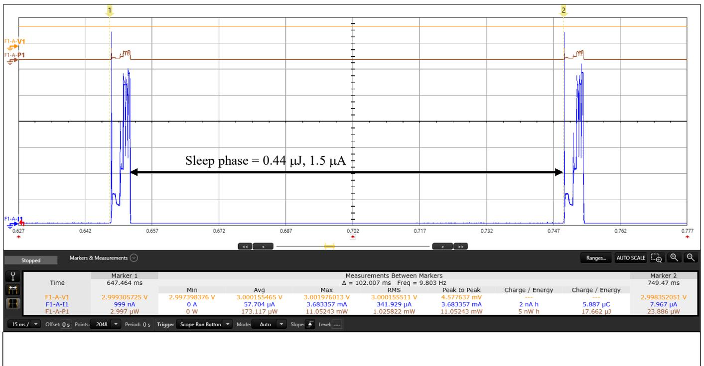
Fig. 7. ADV (ADV\_NONCONN\_IND) event with sleep phase for Toshiba TC35678 device
