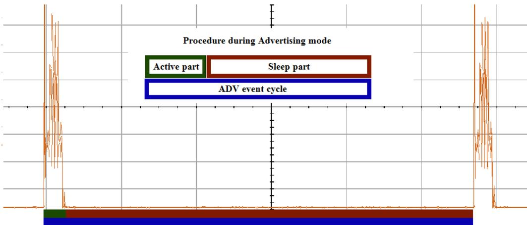
Fig. 4. The ADV event cycle consists in active and sleep parts
