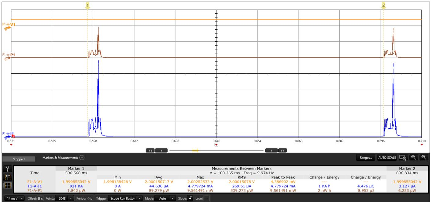
Fig. 10. Energy of Keep Alive connection. NXP QN9080 device (2 V, 100 ms)
