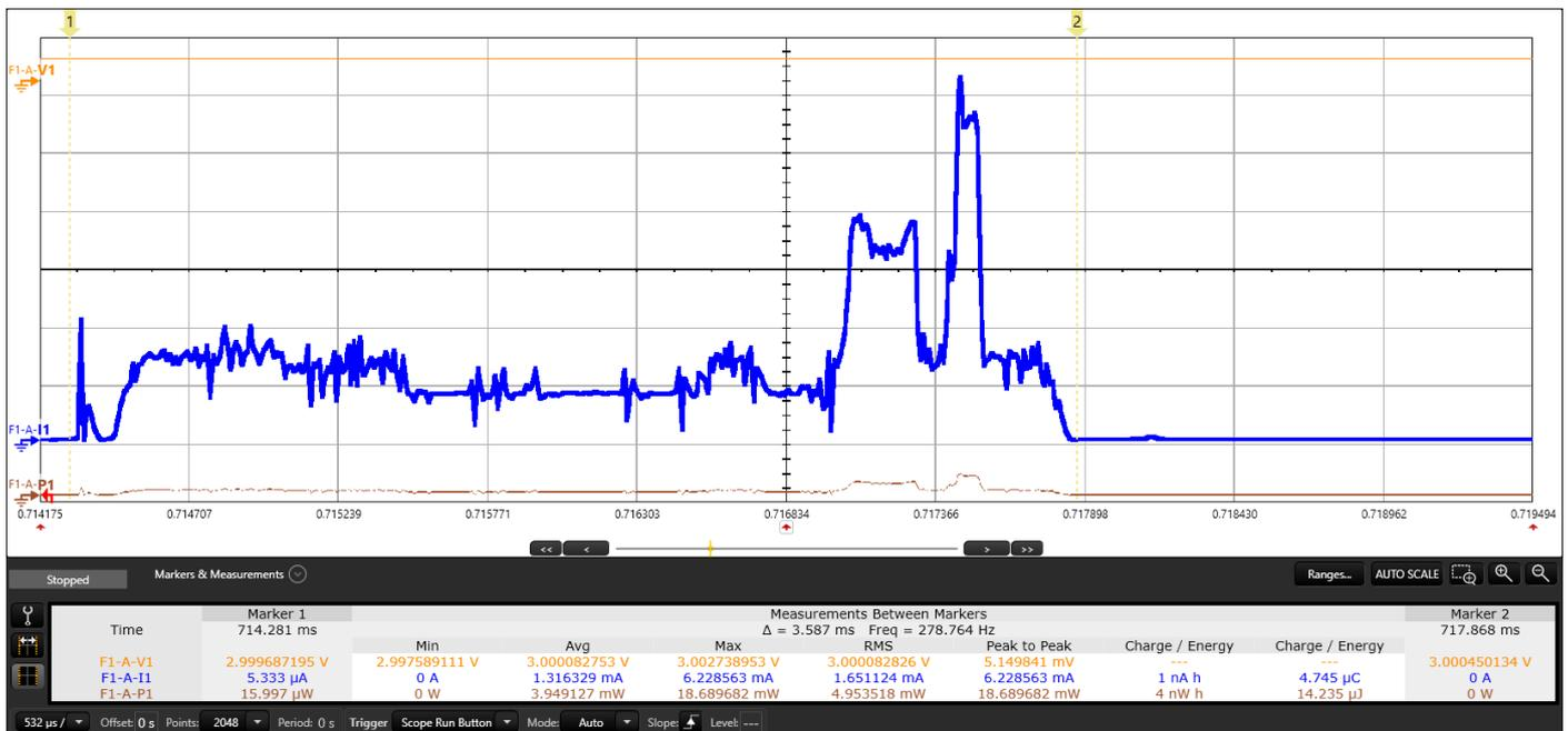
Fig. 14. Energy of Keep Alive connection. EM9304 SD (3 V, 100 ms). Zoom on active part
