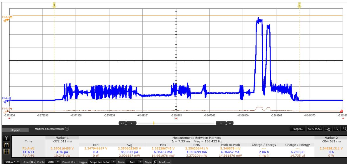
Fig. 17. Energy of Keep Alive connection. Dialog DA14581 device (2.35 V, connection interval of 100 ms). Zoom on active part
