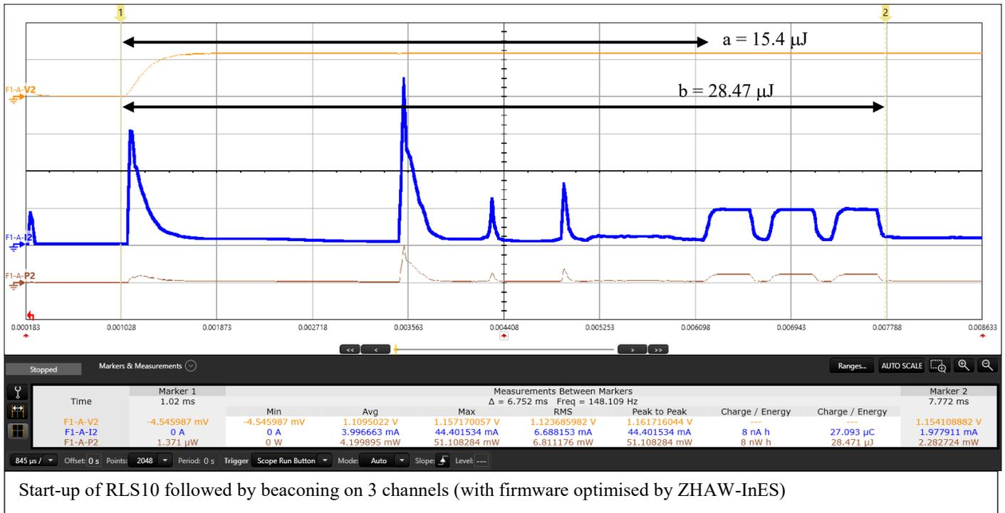
Fig. 1. Energy at different times during Startup & ADV\_NONCONN\_IND (μJ)
