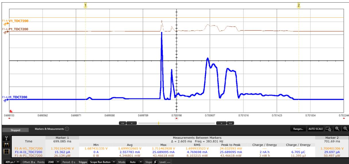
Fig. 13. Energy of Keep Alive connection. Cypress PSoC6 revD device (1.7 V, 100 ms). LDO activated. Zoom on active part
