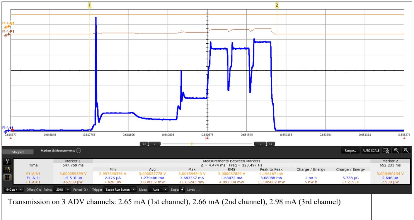
Fig. 6. Active part of ADV\_NONCONN\_IND event for Toshiba TC35678 device
