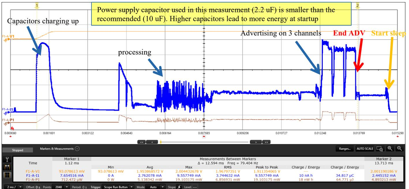
Fig. 3. EM9304 (@ 2 V). Start-up time/energy incl. ADV\_NONCONN\_IND 64.7 $\mu\text{J}$ /12.6 ms (end of ADV) 70.3  $\mu\text{J}$ /14 ms (until Start sleep)
