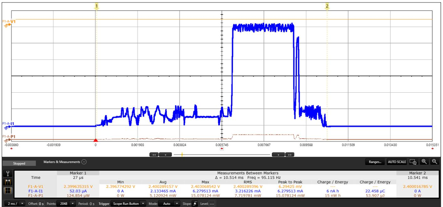
Fig. 16. Energy of Keep Alive connection. Dialog DA14581 device (2.35 V, connection interval of 4000 ms). Zoom on active part
