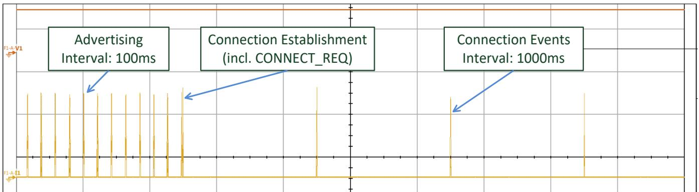
Fig. 8. Example of connection establishment
