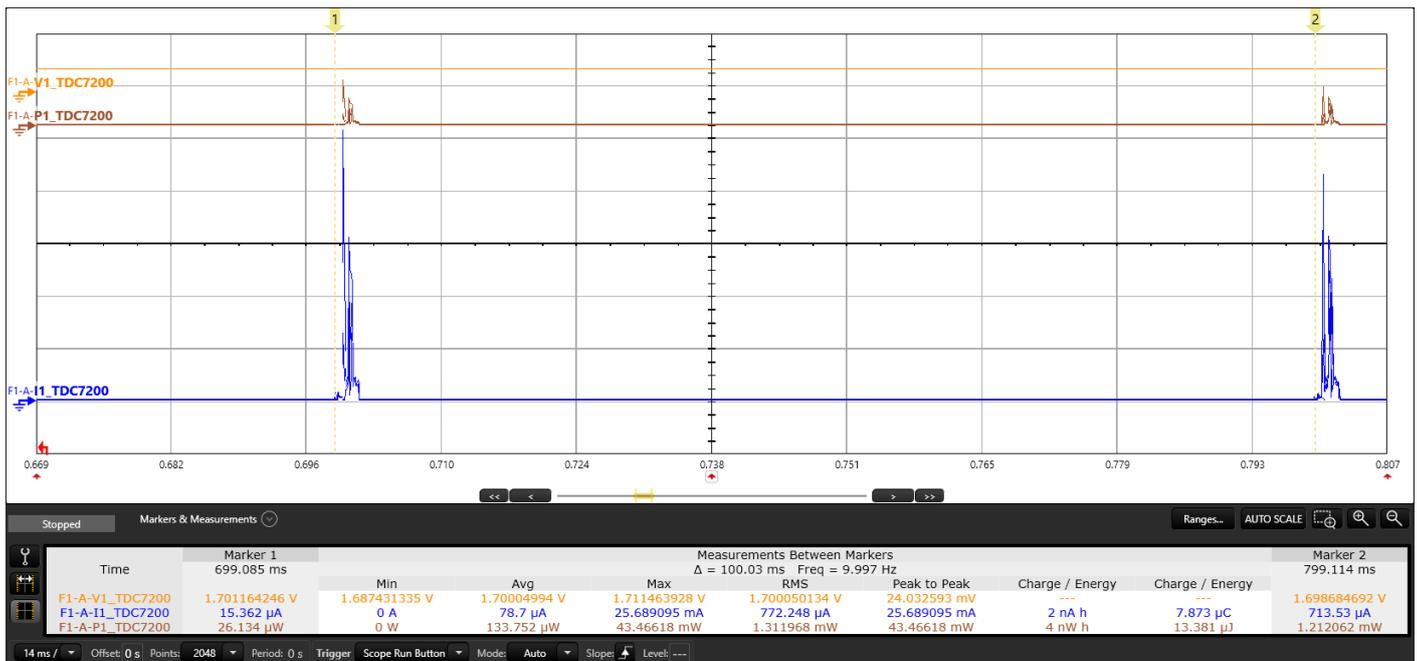
Fig. 12. Energy of Keep Alive connection. Cypress PSoC6 revD device (1.7 V, 100 ms). LDO activated
