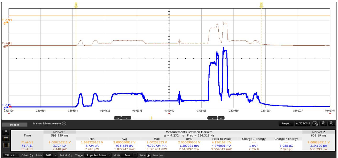
Fig. 11. Energy of Keep Alive connection. NXP QN9080 device (2 , 100 ms). Zoom on active part. RX followed by TX can be clearly seen
