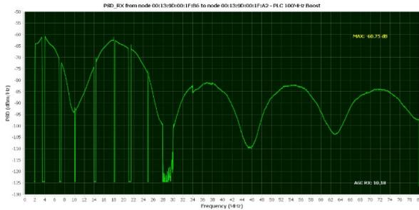
Figure 4: Communication channel middle floor to gateway in shaft head (middle distance)
