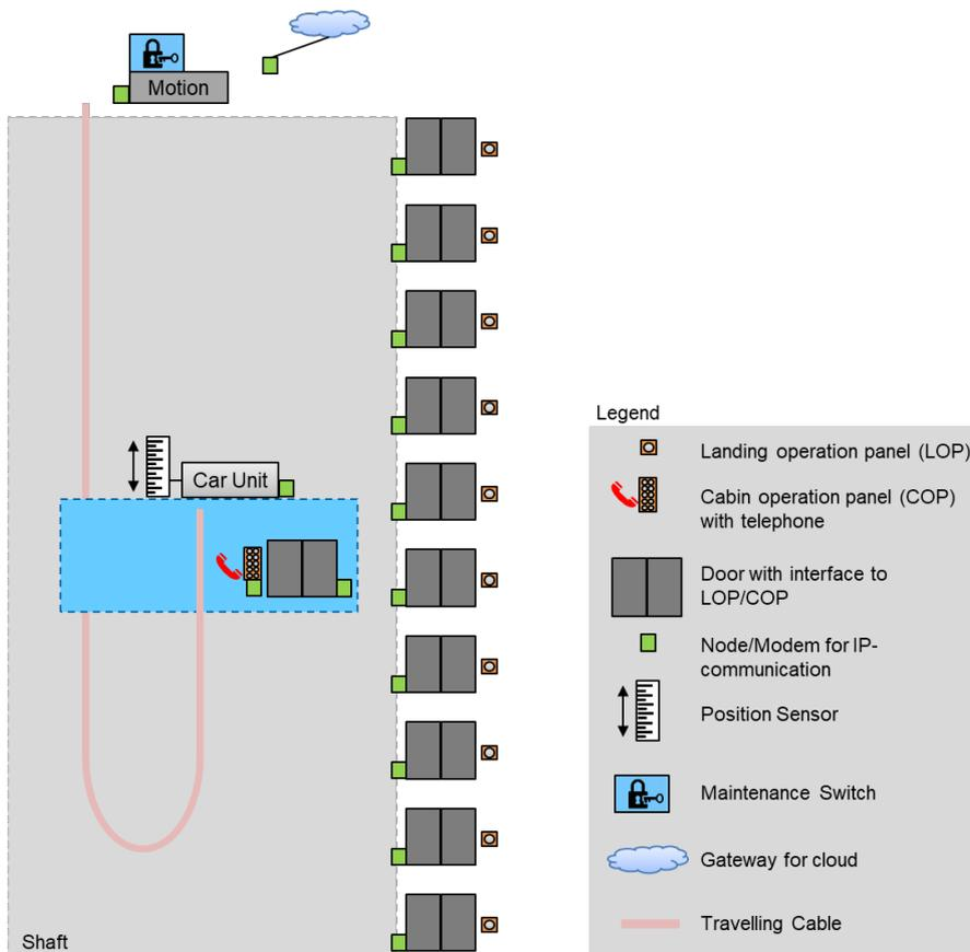
Figure 1: Network of an elevator, green squares represent IP nodes
