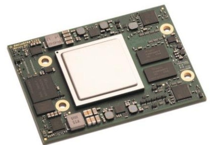
The Zynq Ultrascale+ from Xilinx is an SoC (System on Chip) with programmable logic and multiple processors on a single chip.
