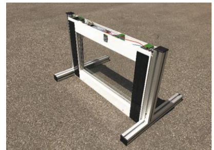
Demonstrator of the autonomous and autarkic ventilation system
