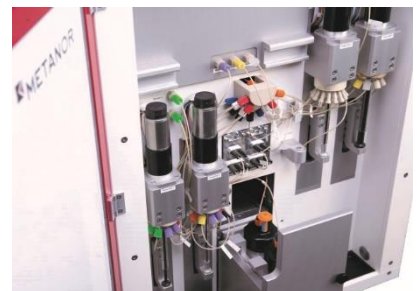
Online-Bacteria-Analyzer with pump system
