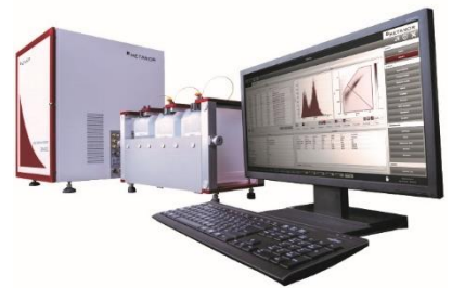
Online-Bacteria-Analyzer with Flow-Cytometer, chemical tanks and user interface
