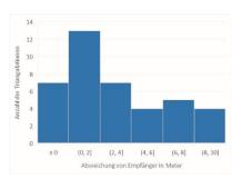
Positional deviation of a triangulation with two meters of space between the antennas in a room with sources of interference. A value equal or less than zero means that no triangulation was possible.
