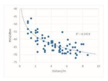
Relationship between signal strength and distance in a room with sources of interference, in which a function is fitted
