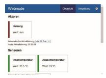
The developed web front-end displays the state of the switched outputs and the values of the connected sensors. The device settings can also be managed with the front-end.
