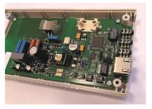
A view on the hardware which was designed by the industrial partner. It features an ARM Cortex-M3 CPU with 72 MHz, 64 kB SRAM and 256 kB Flash memory.
