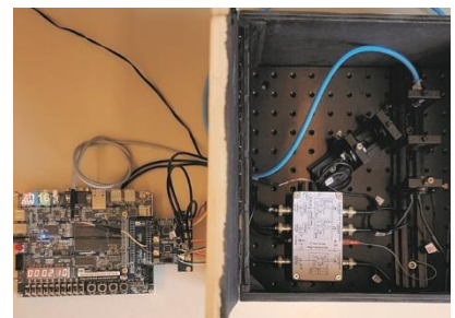
Laboratory setup of the oxygen sensor with the FPGA-board (left) and the optical setup in the black-box (right).
