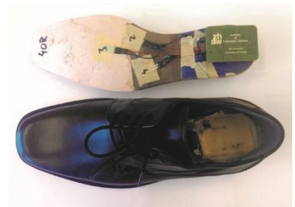
Overview of the finished product. On the top, the sole with the built-in sensors and the circuit board is visible. On the bottom, the shoe with the cavity in the heel is shown.
