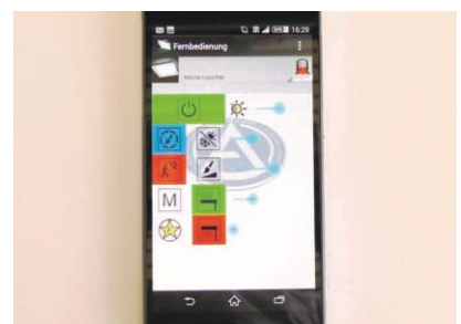
The developed application for Android. The application allows configuration and remote control of the LED lamp.
