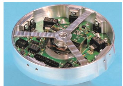
The motor controller was developed in a compact form factor. The figure shows the power electronics and the optical positional sensor mounted inside the aluminum housing.
