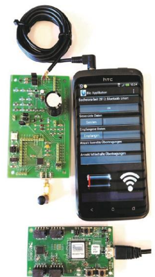
The smartphone communicates via the audio jack with the developed print. This establishes a wireless connection via Bluetooth smart with the evaluation board.
