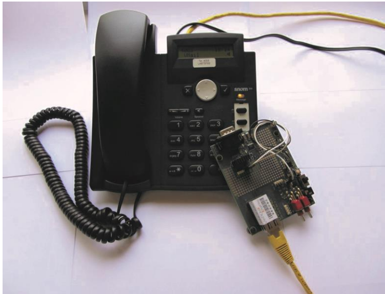
The embedded webserver XPort Pro and a VoIP phone.
