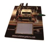
The development kit LM3S9B96, a product out of the Luminary Micro factory, consists of a 80 MHz Cortex-M3 Controller with 256 KB Flash and 96 KB SRAM, as well as a Ethernet connection and an audio codec.
