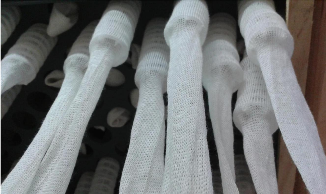
Packing of Watergy direct contact desiccant to air heat exchanger
