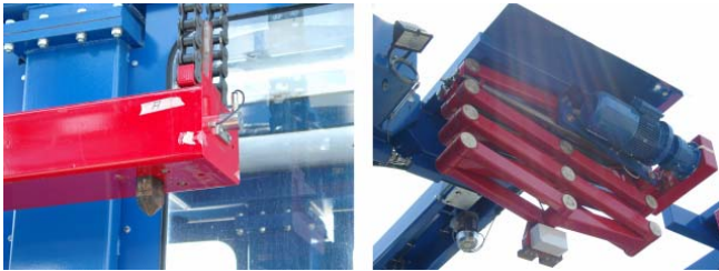
Fig. 3. Twist lock (at the bar) and scissor gripper
