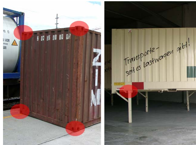
Fig. 2. The container fittings at an ISO (left) and swap body container
