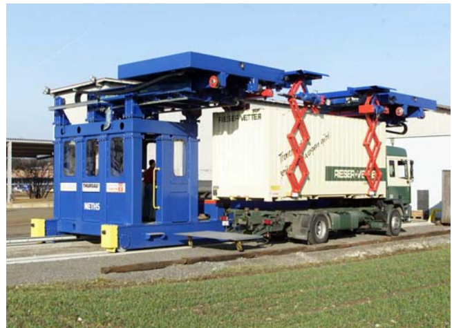
Fig. 1. The container manipulator NETHS handling a swap body container
