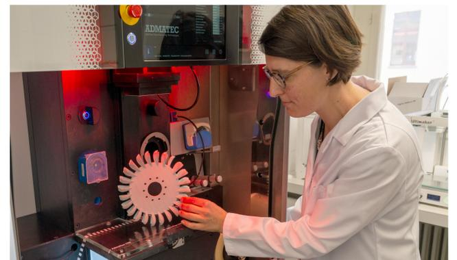
Additive manufacturing using DLP technology
