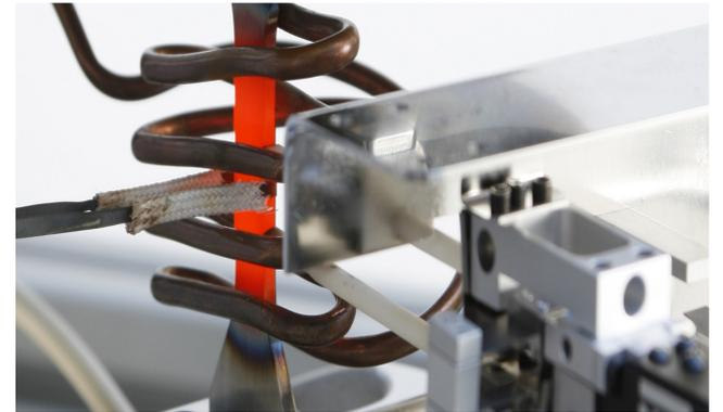
Thermomechanical tests on aerospace components
