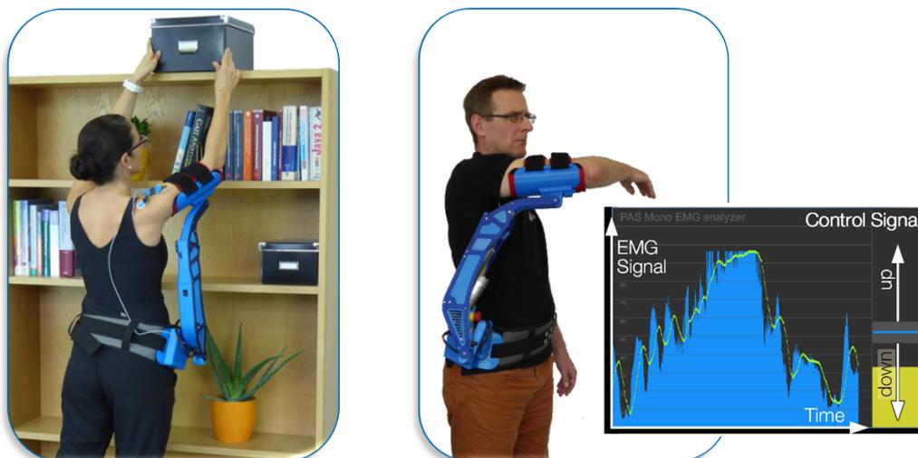
The PAS assists the patient in moving the arm against gravity but without replacing the existing muscle forces. In order to successfully cope activities of daily living, the PAS has to be completely portable, whereas a therapy device can be stationary. Besides patient specific adaptability ease of use, low weight and an appealing design are essential for the acceptance of a PAS.
