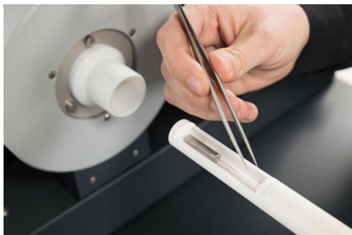
Fig.2: Sample preparation in AlO 2 holder.
