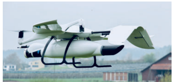
Wingcopter in hover flight - Two swivel motors provide the thrust in cross-country flight
