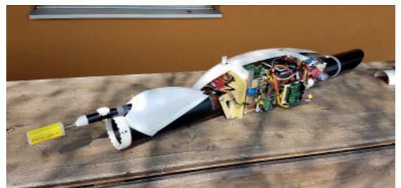
Sensorpod with removed side panel - under the panel are various other sensors, batteries and measurement electronics
