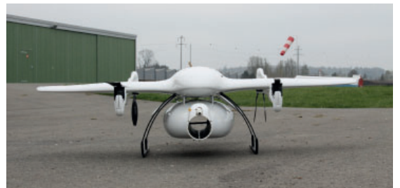
Measuring pod with open flow tube and visible measuring section of the optical CO 2 sensor
