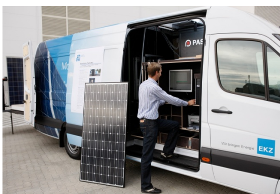
Figure 1: The Swiss Mobile Flasher Bus in operation. The Bus is equipped with a high accurate SunSim Flasher from Pasan and five different reference modules of different technologies on board. (Image source: Photon 2009)
