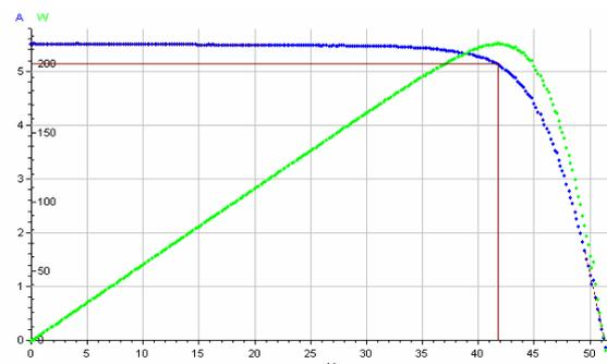
**Figure 4:** Measured current/voltage and power/voltage characteristics by the SMFB yield an STC power of 214.6W of the HIT cr. silicon solar module (PV Module type: Sanyo HIP215, serial no. 8ZEA08483, manufactures nominal power 215W class A). The total IV sweep time of 120ms was subdivided into 15 single flashes according to the Pasan standard splitted flasher
