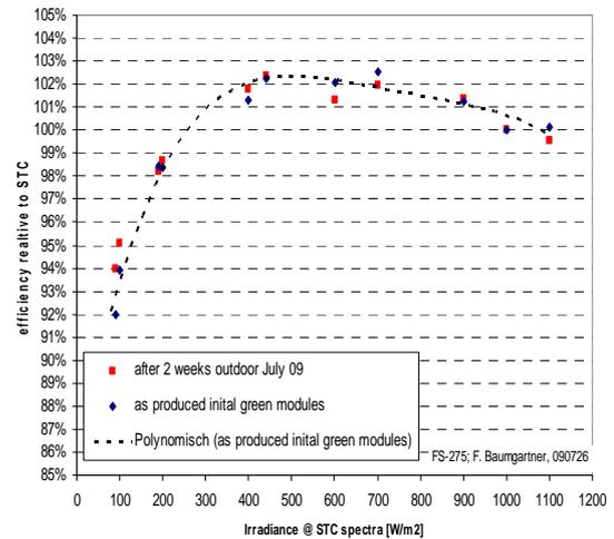
**Figure 6:** Measured module efficiency of a CdTe type Module (FS 275, First Solar) at low irradiance. The values for modules as produced are nearly the same as for modules exposed to outdoor conditions for 2 weeks in July 2007 – OC condition)
