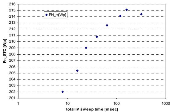
**Figure 5:** Measured STC nominal power of an HIT cry Si solar module versus total IV sweep time using the standard splitted/multi-flash measurement mode of the PASAN SunSim 3c flasher. (Module type: Sanyo HIP215, 8ZEA08483, nominal power 215W class A)
