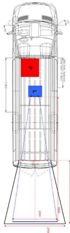
**Figure 1:** Top view of the Swiss Solar Flasher Bus with an overall length of the bus of 10m with a stretched
