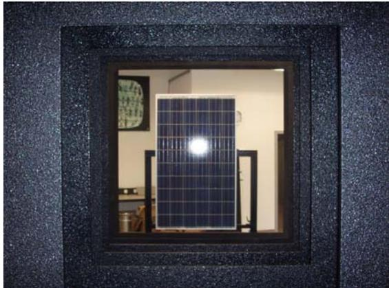
**Figure 3:** Top view of the DUT (measured PV module SM 230, dimensions 1.6m x 1m) through internal light tunnel of the SMFB. The orientation of the module plane is tested using the reflection of a laser light between DUT and the lamp housing.
