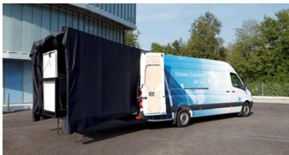
**Figure 2:** The Swiss Solar flasher bus is equipped with a high-quality flasher Sun Simulator 3c from PASAN (PV-module dimensions 2m x 2m). The movable platform in the rear part of the SMFB is covered with a black cloth
