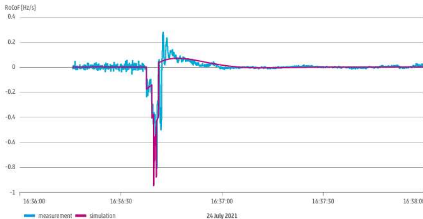
Figure 24: Simulation results (ROCOF) of the single busbar model and comparison with real PMU measured value (La Cereal).
