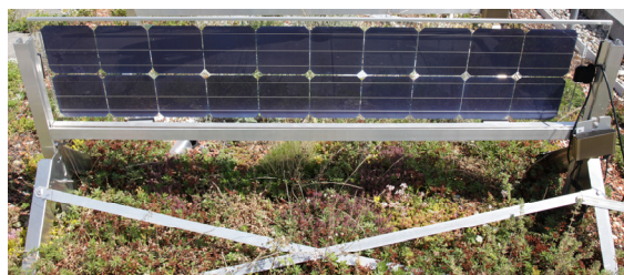
Figure 4 Custom-made 20 cell bifacial module with MegaCell monocrystalline n-type silicon cells. The average STC-power of the four modules measured is 82.2 W on the front side and 71.6 W on the rear side.
