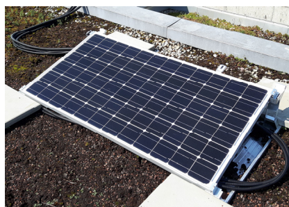
Figure 5 Monofacial south facing (25° azimuth, 16° tilt angle) monocrystalline Silicon reference module of the manufacturer Hareonsolar with a measured STC power of 203.3 W.
