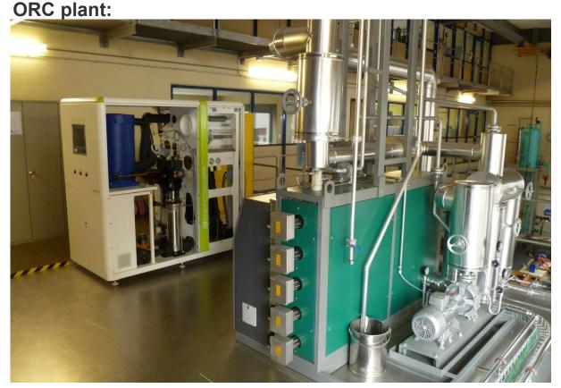
An ORC (Organic Rankine Cycle) process is a steam power cycle (Clausius-Rankine cycle) which is operated with an organic fluid. The process can be operated with less overheating in comparison to water and is therefore suitable for low temperatures. This is made possible by the positive slope of the vapor curve of the organic fluids. ORC systems convert waste heat from industrial processes into electrical energy at a temperature range of approx. 100 to 450°C with an efficiency between 10 and 15%.
