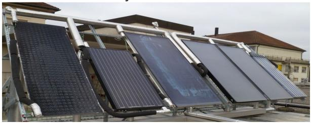
The solar thermal test facility is used for student training as well as research and development. Up to 6 collectors can be installed on the roof of the machine laboratory at the IEFE. The collectors are south facing with adjustable tilt angle. Each collector has separate supply lines, which allows independent operation of the collectors.
